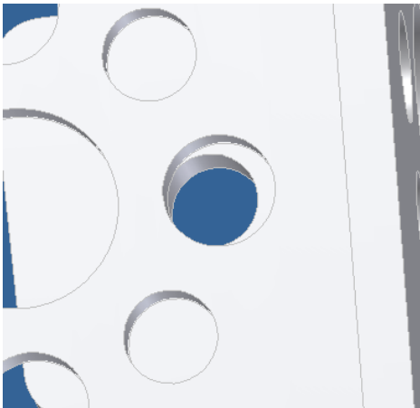
Crooked bars (above) cause the connecting holes (below) to not line up
